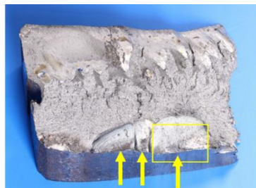
Breakage on the running surface of the wheel through microscopic examination
